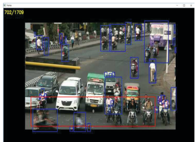
Fig. 7. Violation Detection from Real World Frames
