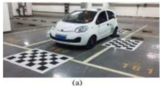
Fig. 12. Camera configurations of prototype vehicle. (a) Cameras calibration
